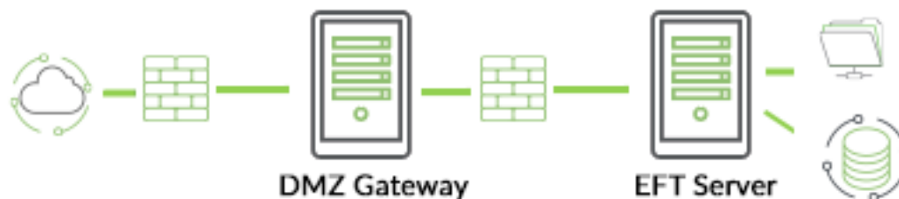
Figure 2 Standalone EFT Server with DMZ Gateway
