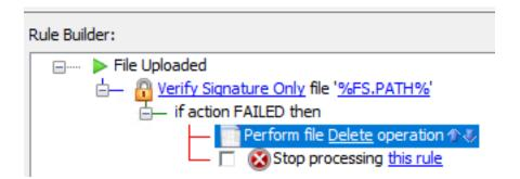
In this example, uploading a file to the server triggers the OpenPGP module to verify the signature on the file that was uploaded. Subsequent actions can be added to the event rule depending on success or failure of the upload.
