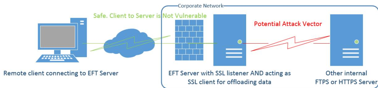
Regarding the Anonymous ECDH denial of service vulnerability, EFT does NOT use ECDH ciphers by default. The EFT application defaults to the following SSL ciphers on the server side:
