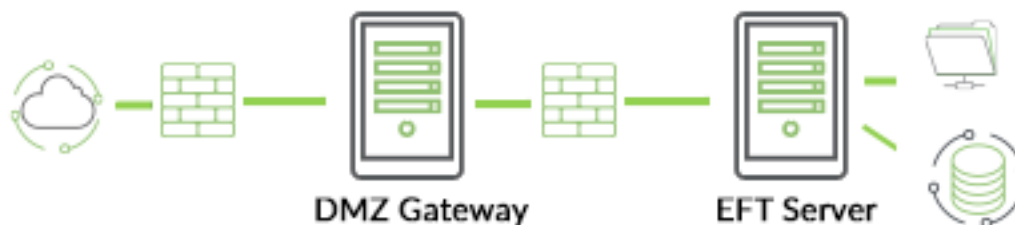
Figure 2 Standalone EFT Server with DMZ Gateway
