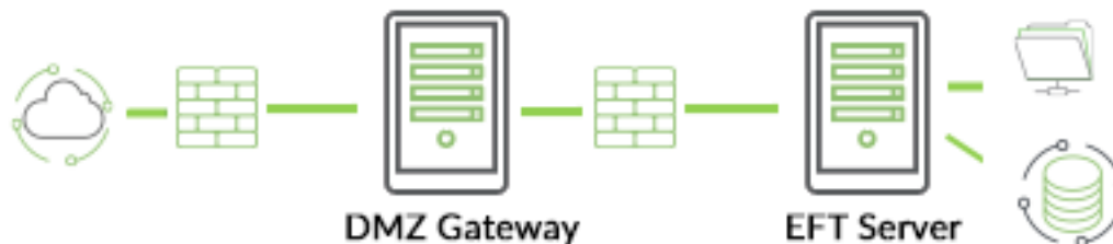
Figure 2 Standalone EFT Server with DMZ Gateway
